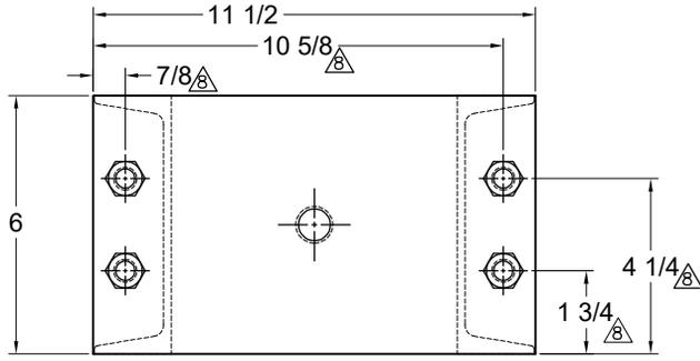
**TYPE ME-3R SPRING ISOLATORS WITH INTERNAL ADJUSTMENT**
